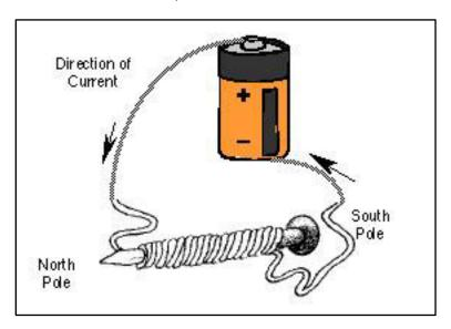
Students should then remove the 60 cm wire from their nail and using the 150 cm wire, they will make 40 winds around the nail and repeat the procedure with the longer wire. First, they should make their prediction. Then, carry out the experiment.
